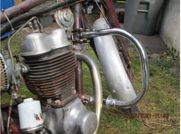
expertly and beautifully welded together by BMOC member Peter Dent. Chromed by Dependable Plating in Burnaby at a cost of \$190, versus \$160 for the powder coating.
