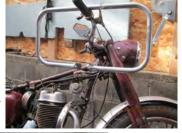
orange peel surface finish. It is paint after all, and applying the powder evenly is not easy.
