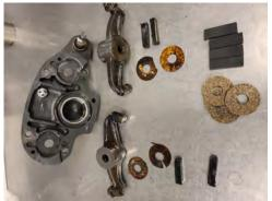
um cam box. Installing new seals was easy — the new ones are rubberized cork washers 70 thou thick, the original cork washers had shrunk to about 25 thou. The rubber wiper pads had also worn and the new ones fit snug against the rockers. I buffed and polished the rockers where the seals go to help with longevity. It all buttoned up nicely and on to recheck the valve clearance.
