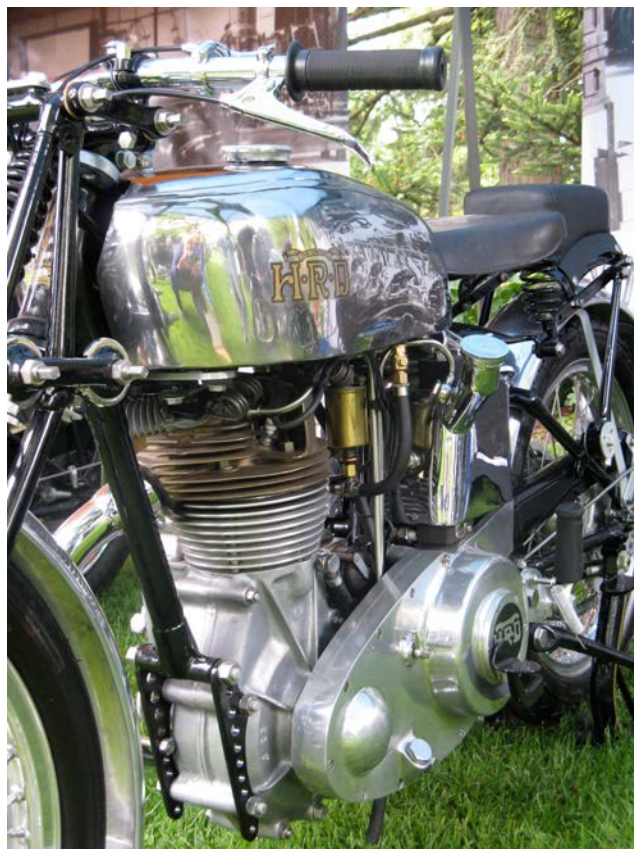
Robert Watson's bronze head '37 TT Replica, a replica of the factory spec racing bike made available to the public.
