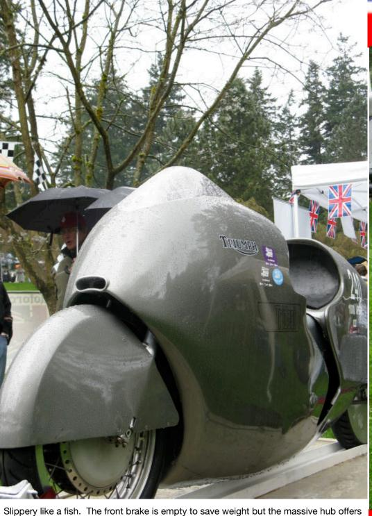
Slippery like a fish. The front brake is empty to save weight but the massive hub offers an aerodynamic edge. A solid wheel would be quicker but is against the class rules so this is as near as Tom can get to one whilst keeping the scrutinisers happy. A world record is all about the details - and nerve, lots of nerve.
